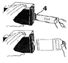
Load the proofing back on the camera and remove the dark slide. Make your exposure.
