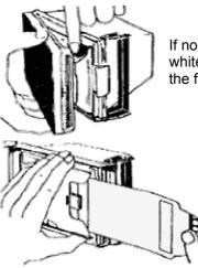
If no yellow tab appears when you pull the white tab: Stop! Do not pull another white tab. Instead, carefully open the proofing back in dim light without disturbing the film pack. Use your finger to make sure the pack does not move.
