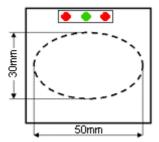
The built-in exposure meter with three LED indicators provides direct throughthe-lens metering. This meter measures the integrated brightness of the image on the focusing screen of the camera.
