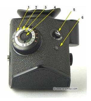
**3.** Without disturbing the film speed setting, rotate the thin silver ring 2 with the f stop sequence on it until the maximum aperture of the lens you will be using is aligned with the red arrow on the film speed portion of the dial. This is necessary to get correct exposure results.
